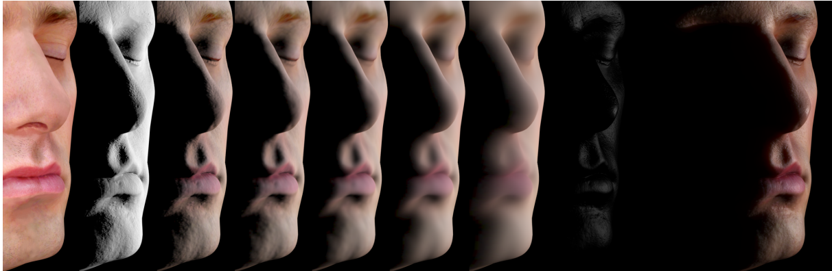
Figure 1: We project multi-layer diffusion profiles onto a sum-of-Gaussians basis to enable realistic rendering of human skin at 30 frames per second on a modern GPU. From left to right: Albedo (1st) and irradiance (2nd) combine to give subsurface irradiance which is then convolved with each Gaussian basis profile (3rd through 7th) and combined in a final render pass with specular (8th) to produce the final image (9th). Convolutions are performed in off-screen 2D textures but shown here mapped onto the face.
